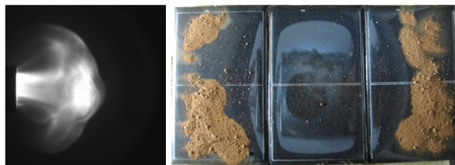
Fig. 1: a) Image of plasma jet in \text{CO}_2 at 5 torr; b) cleaned PV after 20 shots at 1 kV.
